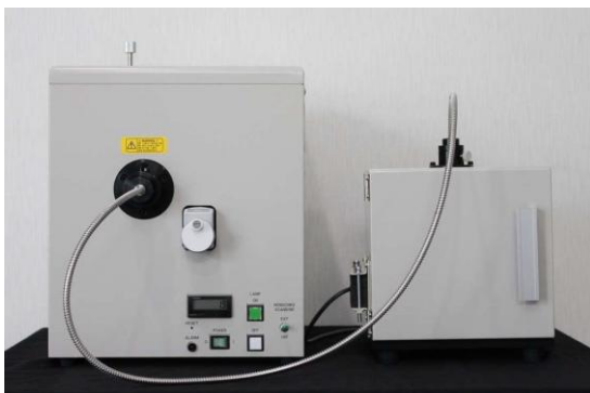
EQE (IPCE) measurement setup (desk top size)
