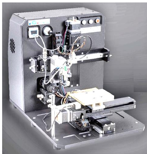
Inkjet coating system for perovskite film coating (film pattern designed on PC controller)
